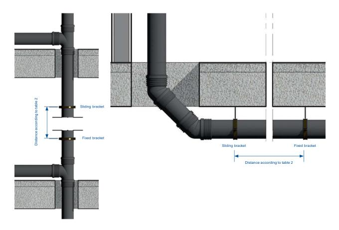
Fig 9: Example horizontal and vertical installation.
