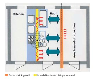
The comparison of the floor plans above demonstrates how good acoustic design in the lower building example can significantly reduce the noise levels to which areas requiring noise protection are exposed.
