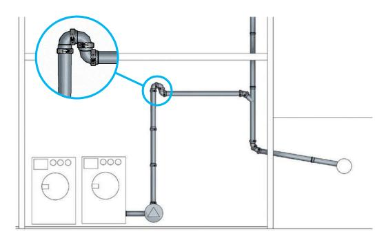
Fig. 12: Tensile resistant connection.
