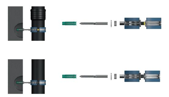
Fig. 10: Low noise bracketing - 21dB(A).
