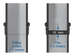
Fig. 8: 10 mm space for thermal expansion.
