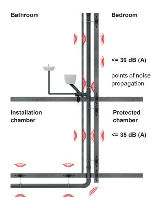
Fig. 5: Example of noise propagation during drainage.
