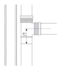
Install a short piece of temporary pipe halfway onto the repair coupler to secure a correct positioning of the rubber seal. Install the free half of the coupler onto the existing pipe and slide the repair coupler completely over the existing pipe.
