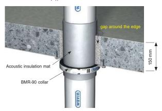
Fig. 20: Straight installation without sleeve / socket up to 160 mm.
