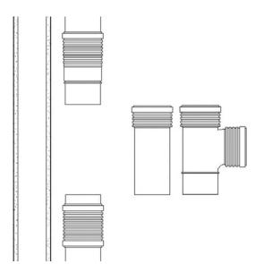
**7.** Push the socketed of the branch or pipe on to the long socket.
