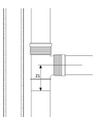
3. Install close to the two pipe ends wall plates for the fixed-point brackets and mount the threaded rod and back part of the brackets. When fixating the repair couplers with tensile resistant clamps this step can be skipped.
