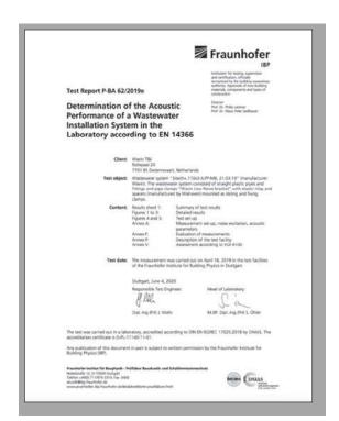
In studies conducted at the Fraunhofer Institut für Bauphysik (Fraunhofer Institute for Building Physics), Stuttgart, Wavin SiTech+ has proven optimal sound absorption. The tests were performed in a laboratory accredited by the German Accreditation System for Testing (DAP, file no. PL-3743.26) according to standard EN ISO/IEC 17025.
