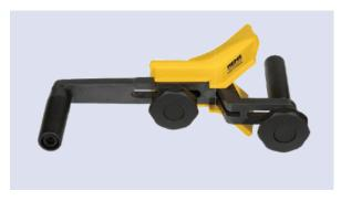
For connections to Wavin SiTech+ fittings or sockets the pipe end needs to be chamfered. Its is recommended to chamfer over a length of 5 mm under a 15 degrees angle. This can be done by using standard chamfer tooling.
