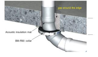
Fig. 21: Straight installation with / without sleeve / socket.
